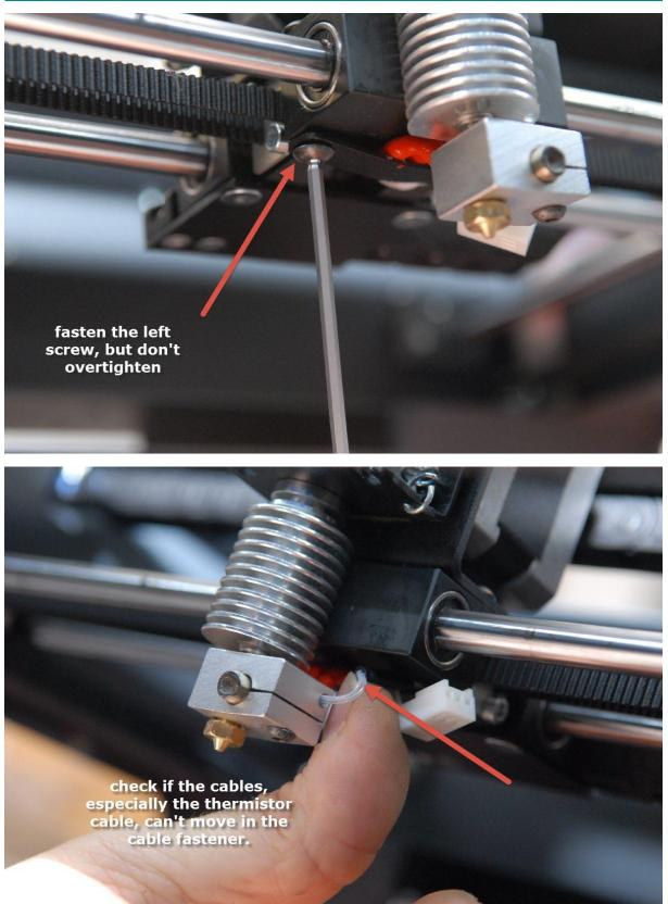
You can fixate the thermistor in the hole with a little piece of kapton, see the end of this manual.
