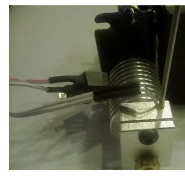
Push the Kapton completely in. It forms a "prop" which holds the thermistor better and keeps the temperature measuring more stable. It is easy to remove.
