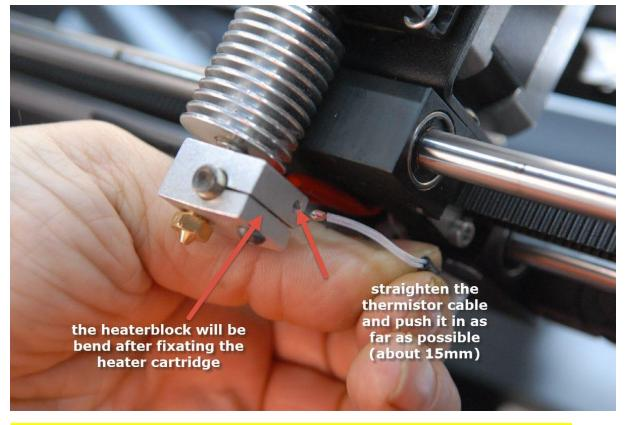
Be sure to use the hole on the right side for the thermistor, NOT the original E3D shallow hole on the backside!
